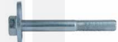
13 Camber Bolt - LTV Part No: 91114A2544 Size: M14 x 1.5 x 115
