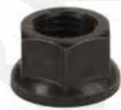
76 Wheel Nut Plain A/F 27 - 1210 Part No: 99120A9035 Size: M20 x 2.5
