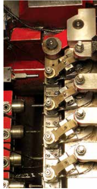
Multi station header
